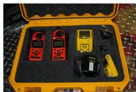
To fully assess the atmospheric hazards present and evaluate the effectiveness of ventilation efforts, the unit is equipped with several monitors. In addition to a standard 4 gas monitor that measures O<sub>2</sub>, CO, H<sub>2</sub>S, and LEL, the unit
